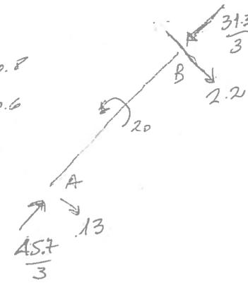
$$\begin{aligned} N_A &= \frac{47}{3} \times 0.8 + 45 \times 0.6 \\ &= \frac{45.7}{3} \text{ kN} = 15.23 \text{ kN} \\ V_A &= \frac{47}{3} \times 0.6 - 45 \times 0.8 = 5.1 \\ N_B &= \frac{49}{3} \times 0.8 + 4.5 \times 0.6 = \frac{31.3}{3} \\ &= 10.4 \\ V_B &= \frac{49}{3} \times 0.6 - 4.5 \times 0.8 = 2.2 \end{aligned}$$
