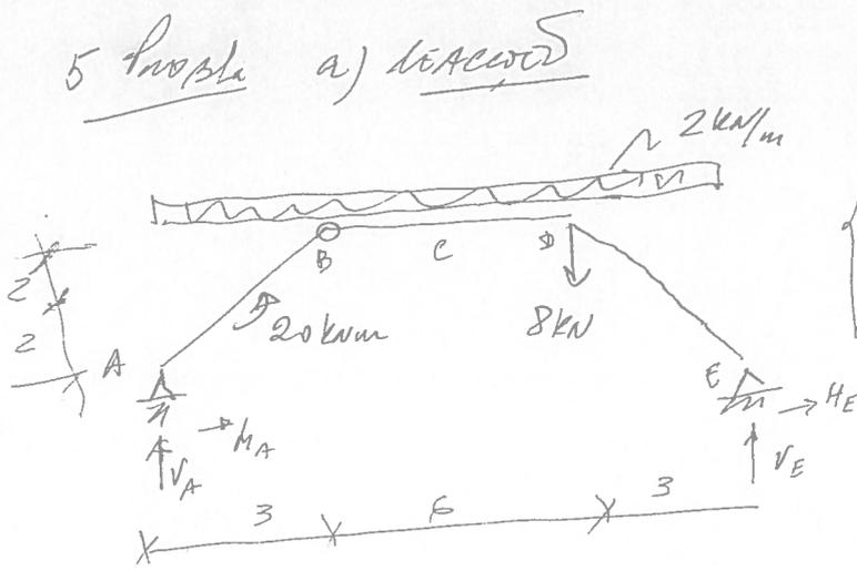
$$\begin{aligned} \sum F_v &= V_A + V_E - 2 \times 12 - 8 = 0 \rightarrow V_A = \frac{47}{3} \text{ kN} \\ &= 15.667 \\ \sum F_h &= H_A + H_E = 0 \\ \sum M_A &= V_E \times 12 + 20 - 8 \times 9 - 2 \times 12 \times 6 = 0 \rightarrow V_E = \frac{49}{3} \\ &= 16.333 \\ \sum M_B &= \frac{49}{3} \times 9 + H_E \times 9 - 8 \times 6 - 2 \times 9 \times 4.5 = 0 \\ H_E &= -4.5 \text{ kN} \rightarrow H_A = 4.5 \text{ kN} \end{aligned}$$
